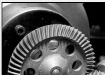
Figure 3—Contact pattern with 120 in.-lbs. of torque. As has been run in a gearbox, the engineer can duplicate the same wear pattern by adding displacement and load. This will generate all the numerical values required for further evaluation.
