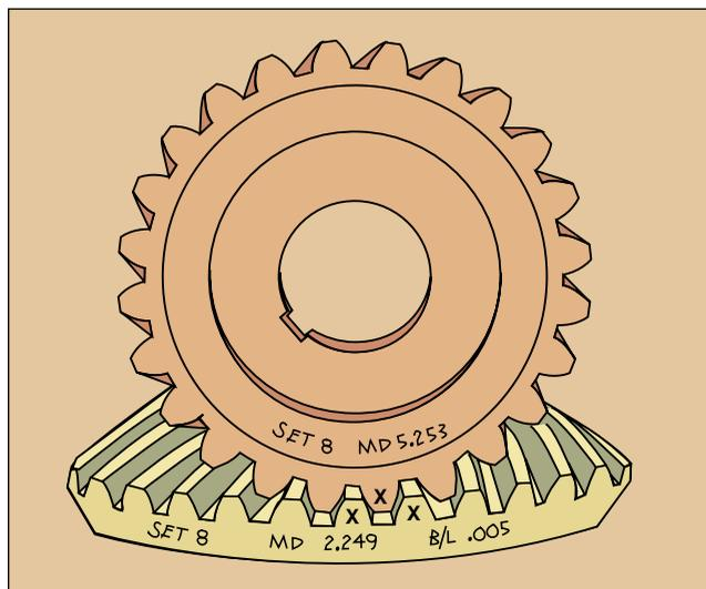
**Figure 3 — Normal backlash in a set of spiral bevel gears is measured perpendicular to the tooth surface at the outer end (heel) of the tooth, using a dial gage.**
