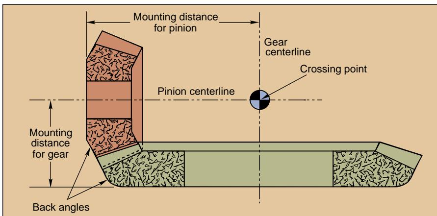
Figure 1 — Mounting distances used for assembling bevel gears.
